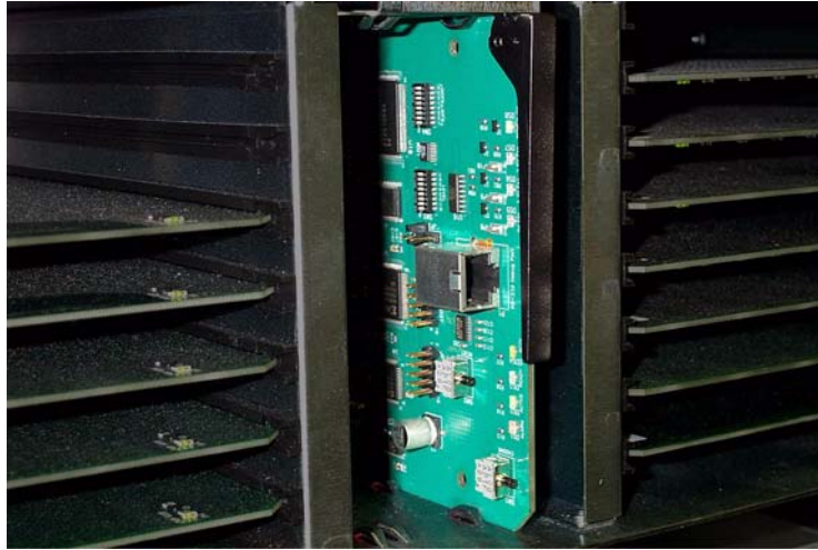
FIGURE 3-4. Crosspoint Board Replacement and Removal
