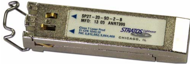
FIGURE 4-16. SP2T - Transmitter module
