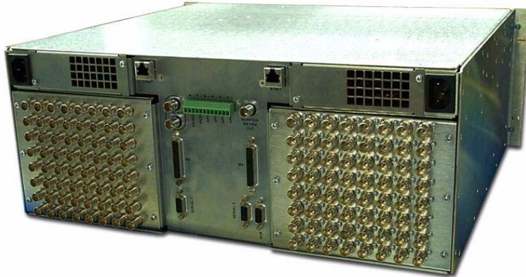
FIGURE 4-22. 64x64 Audio backpanel -- BNC and D-sub connections shown
