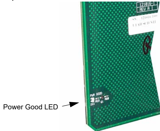
FIGURE 4-11. SD and HD Output Power Good LED
